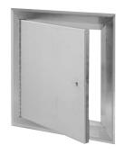
This lightweight, insulated, all aluminum access door is ideal for exterior applications, and also those specific interior applications where corrosion or moisture is a concern. Access to large openings in walls and ceilings is made easy. The aluminum door panel is lined with 3/4" polystyrene insulation.
